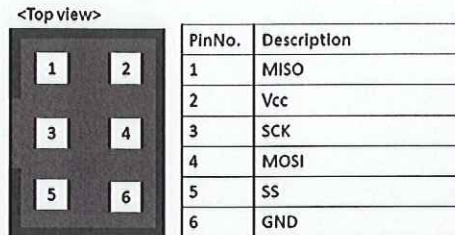
Fig. 2. Pin assignment of the connector. The top view of the connector mounted on the board is shown in the left. The pin assignment is based on the ICSP, however, the RESET pin has been assigned to the SS pin in our design.
